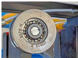
The piping profile fed from a large coil is threaded into the rolling mill from below via a deflection roller shortly before the edge of the slat is formed.
