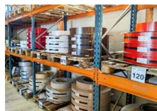
The starting product for slat production is pre-painted aluminium strips in numerous colours.
