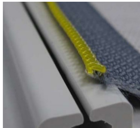
Fig. 2: In order to be able to guide the Zipscreens pulled tightly to the side, their reinforced outer edge features nubs made of a plastic with good sliding properties. They are guided in plastic profiles.
